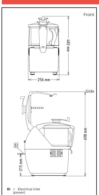
Electric Supply voltage: 600445 (DK55Y2V) 380-440 V/3 ph/50/60 Hz Electrical power max.: 1 kW **Total Watts:** 1 kW Capacity: Performance (up to): 2.5 kg/Cycle 5.5 litres Capacity: Key Information: External dimensions, 256 mm Width: External dimensions, Depth: 415 mm External dimensions, Height:
